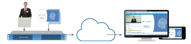
The HD Encoder 2/HDMI can be used as a standalone presentation capture system that encodes video and slides, streams them across the network, and records them for on demand viewing. The video and slides are recorded independently as high quality H.264 MP4 files up to 1080p and can be uploaded automatically to a NAS or other network storage, where it can be integrated with Encoded Media Video Library.
